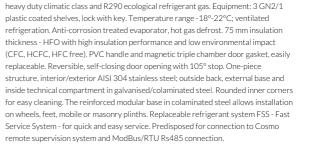
Smart 700 refrigerated cabinet, 1 door. Plug-in refrigeration unit, C energetic class, 5
